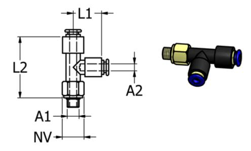
Ext. hose diameter A2 = 4 mm L1 = 14 L2 = 31.6 NV = 10 Thread A1 = M6
